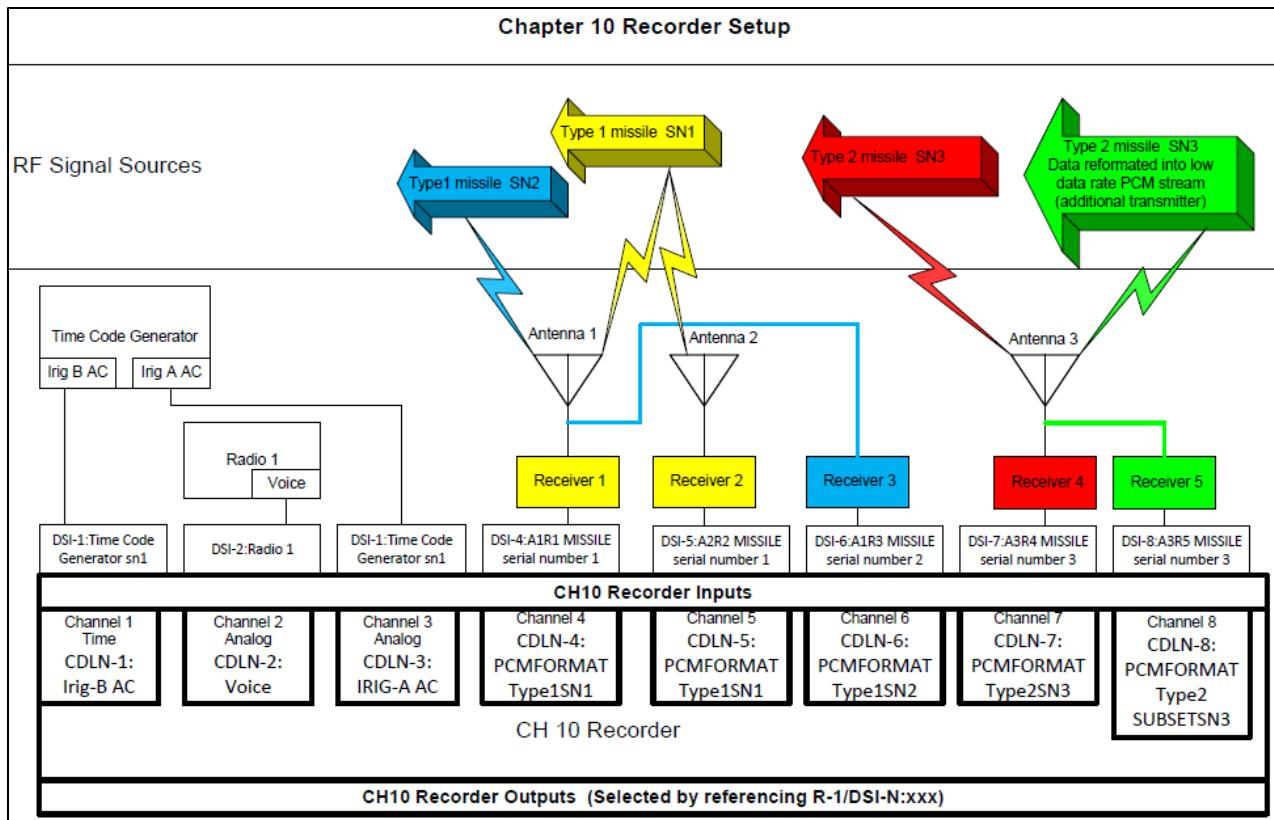
Figure 5-49. Data Source ID-Data Link Name Example
