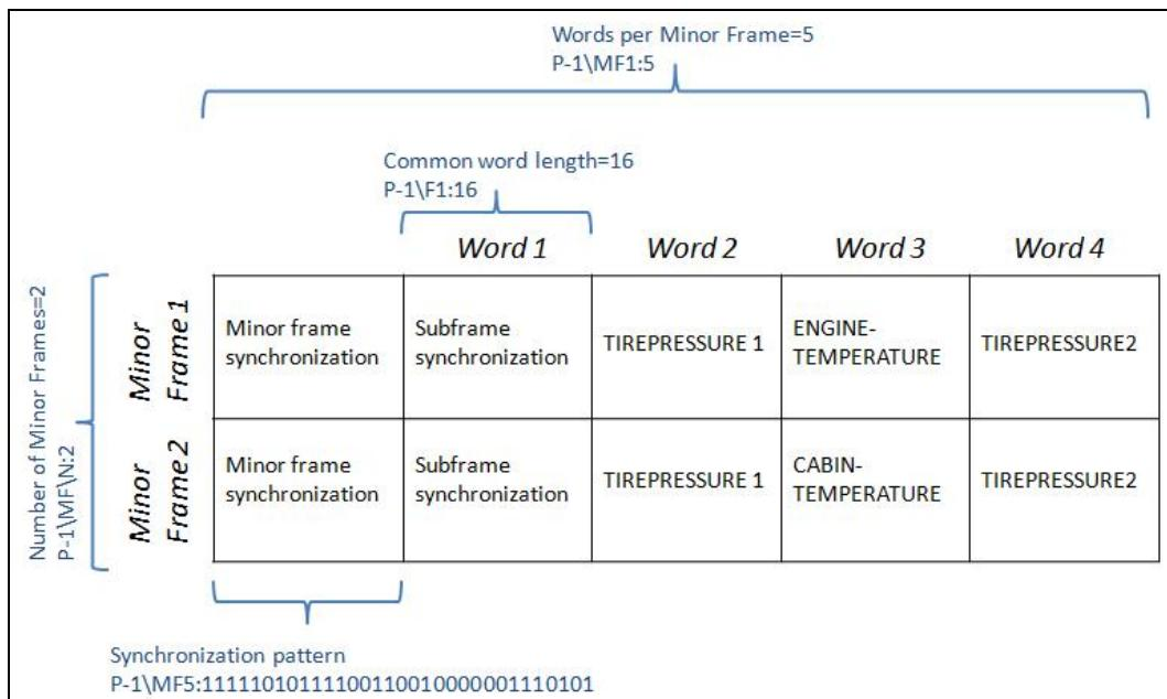
Figure 3-7. Attributes Used to Describe a PCM Format
