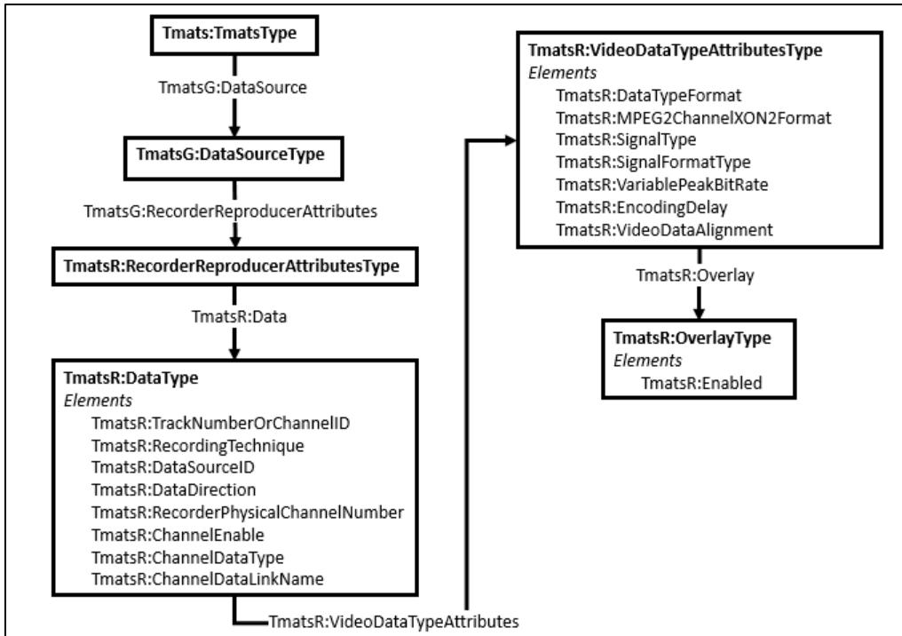
Figure 5-46. R-Group Sample Video Channel Example XML Schema
