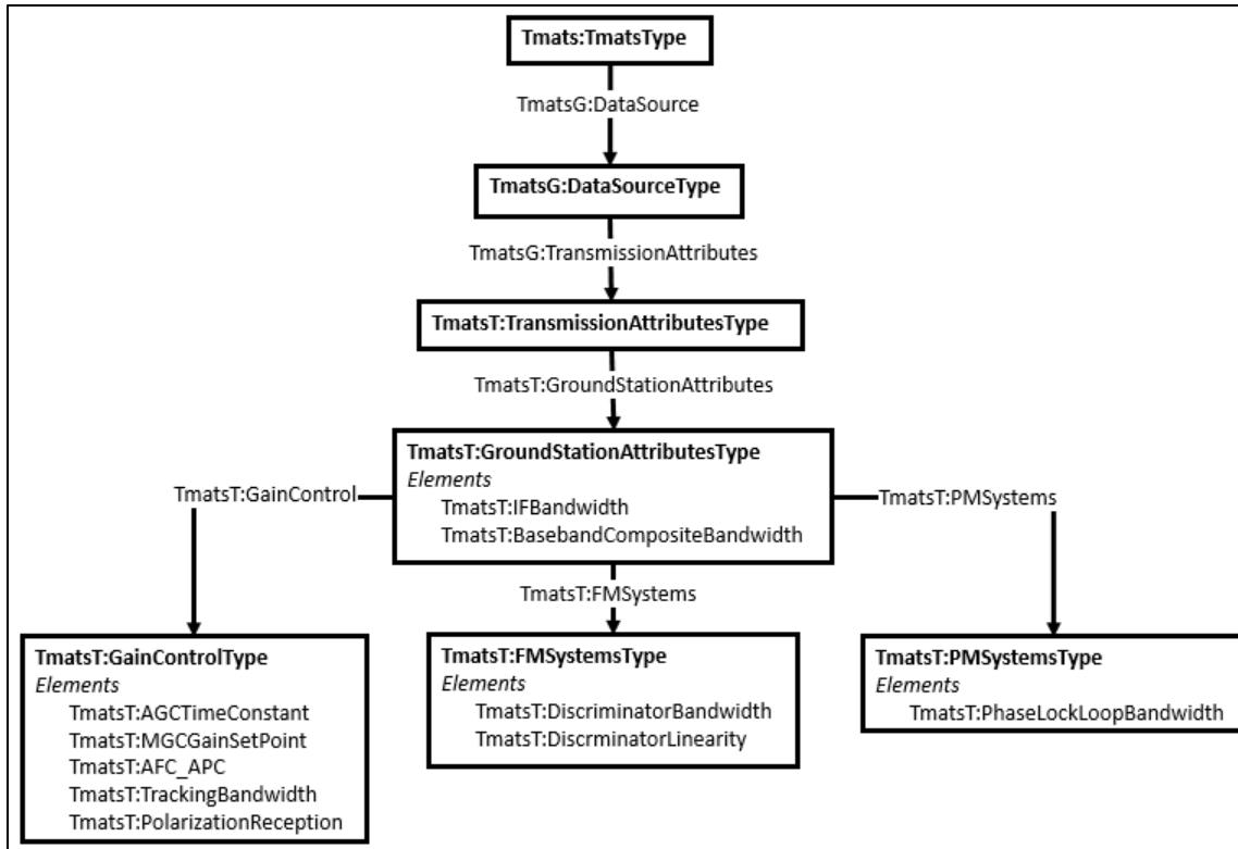
Figure 5-36. Ground Station Attributes Group Example XML Schema
