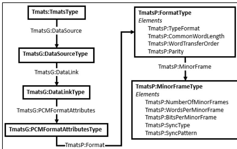
Figure 3-11. PCM Format Attributes Group Example XML Schema
