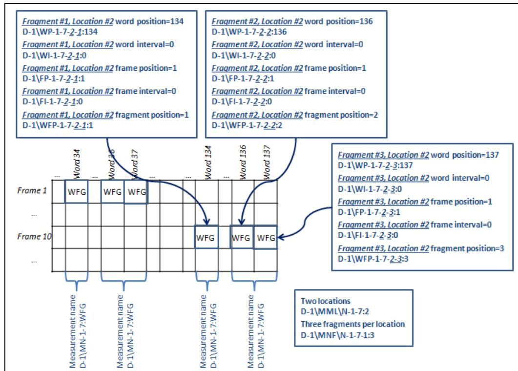
Figure 5-14. Subframe Fragmented Measurement in Multiple Locations (Location 2)
