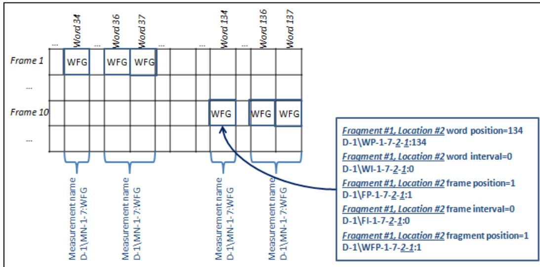
Figure 5-18. Subframe Fragmented Measurement in Multiple Locations
