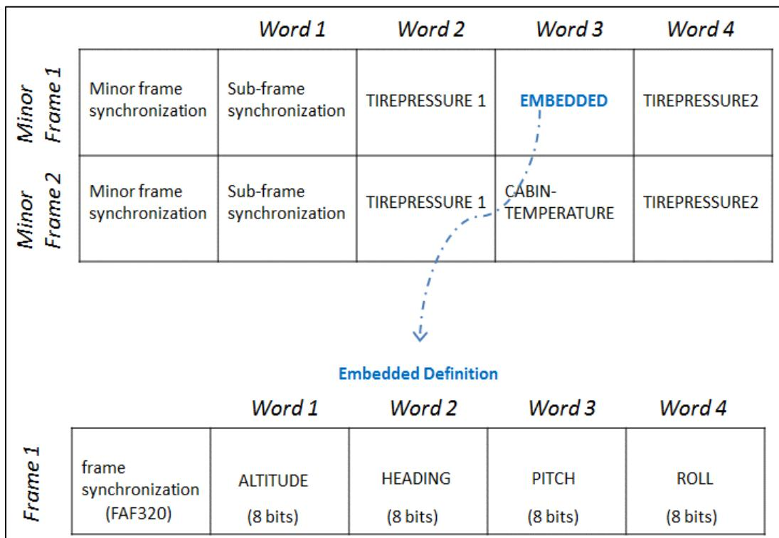
Figure 6-1. Simple Embedded PCM Example
