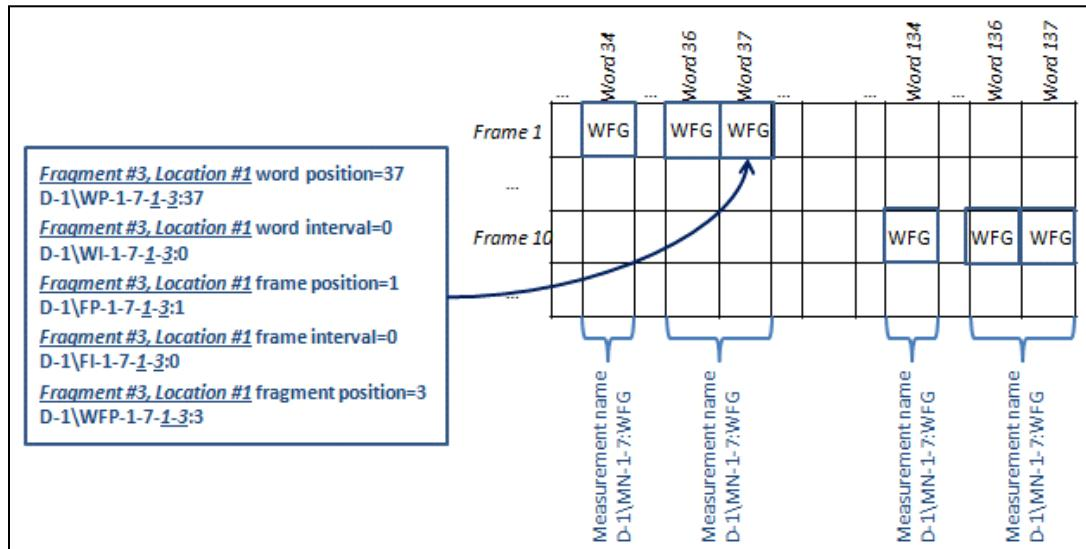
Figure 5-17. Subframe Fragmented Measurement in Multiple Locations
