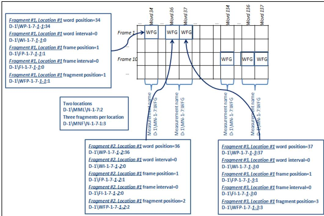
Figure 5-13. Subframe Fragmented Measurement in Multiple Locations (Location 1)
