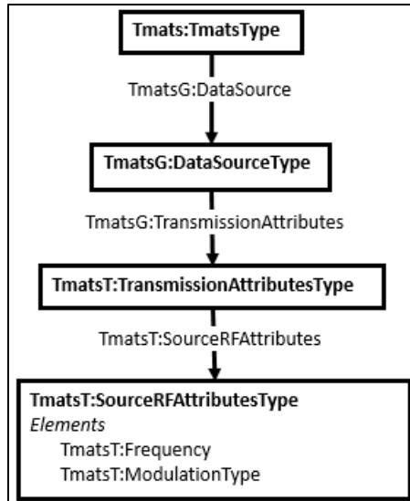
Figure 3-4. Transmission Attributes Group Example XML Schema
