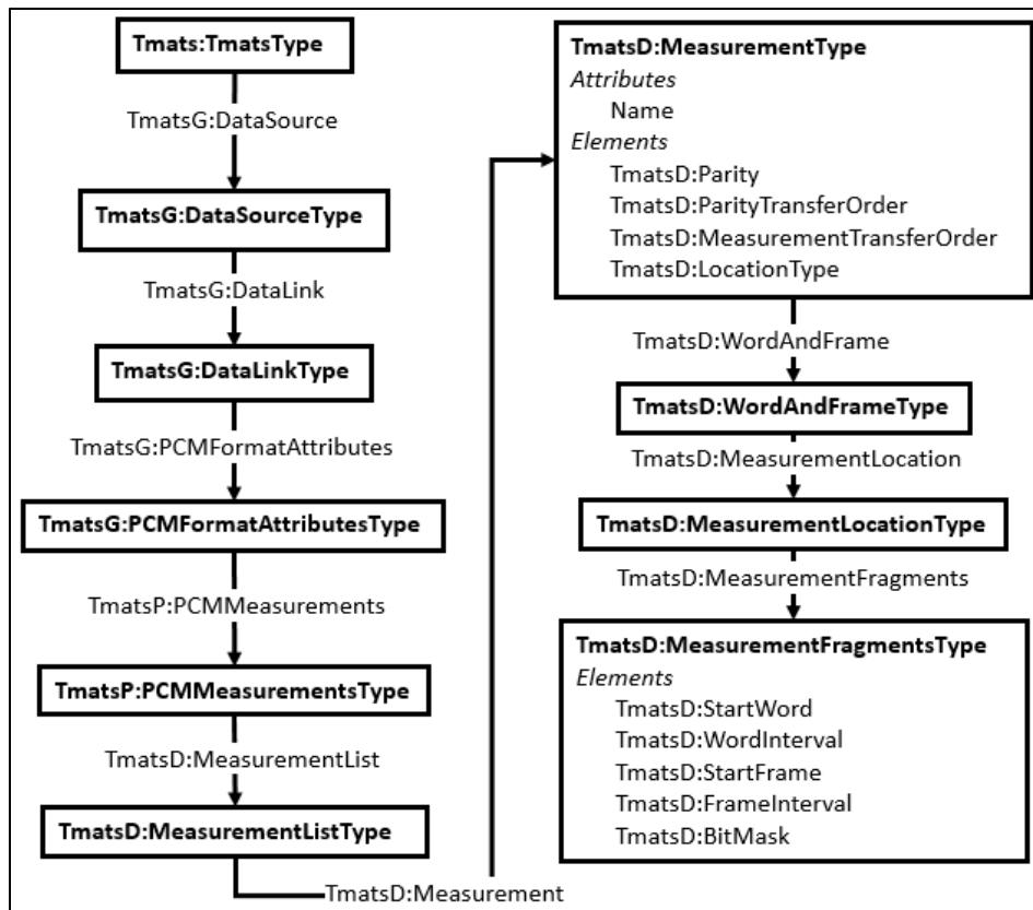
Figure 2-15. “Look and Feel” D-Group Measurement XML Schema
