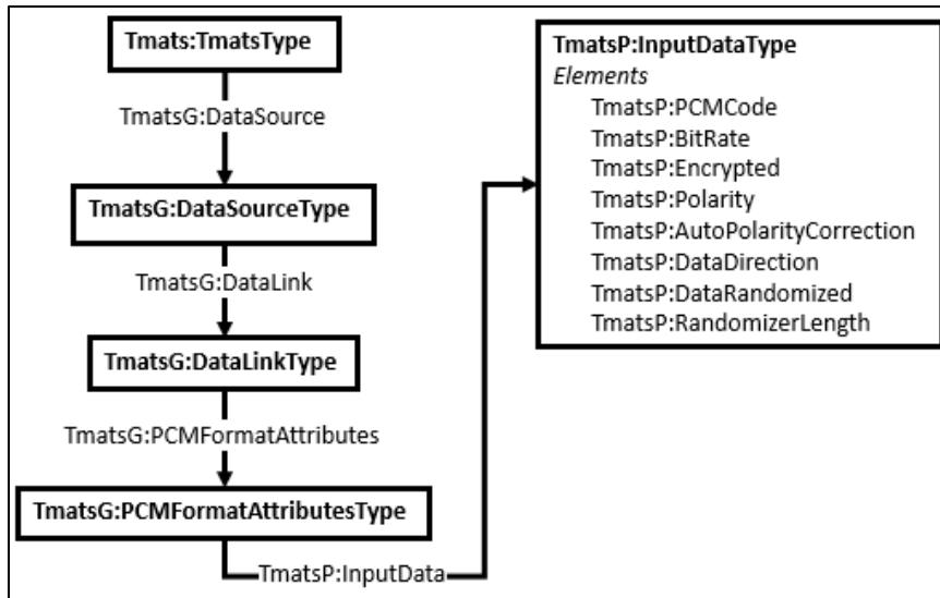
Figure 3-9. PCM Format Attributes Group Example XML Schema
