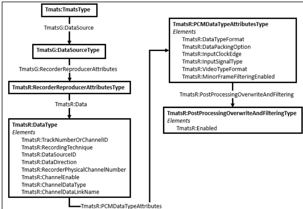
Figure 5-42. R-Group Sample PCM Channel Example XML Schema
