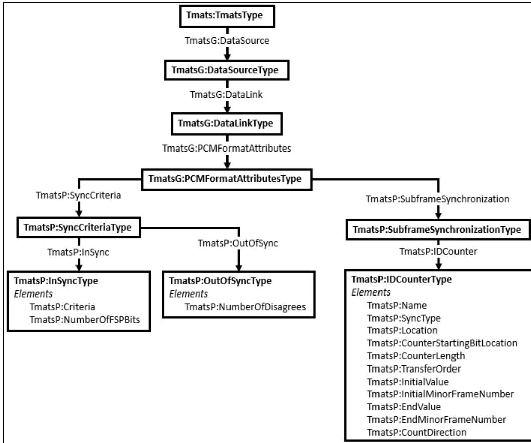
Figure 3-13. PCM Format Attributes Group Example XML Schema
