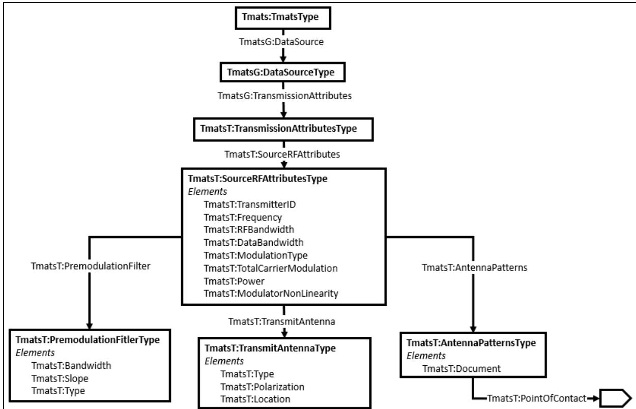
Figure 5-34. Transmission Attributes Group Example XML Schema
