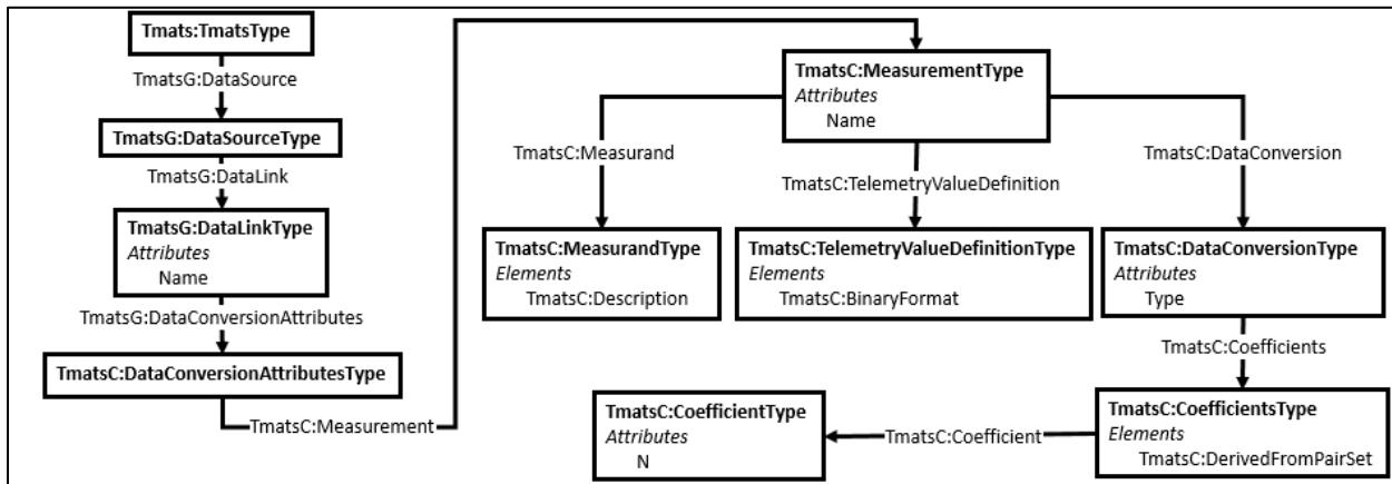
Figure 3-18. Data Conversion Attributes Group Example XML Schema
