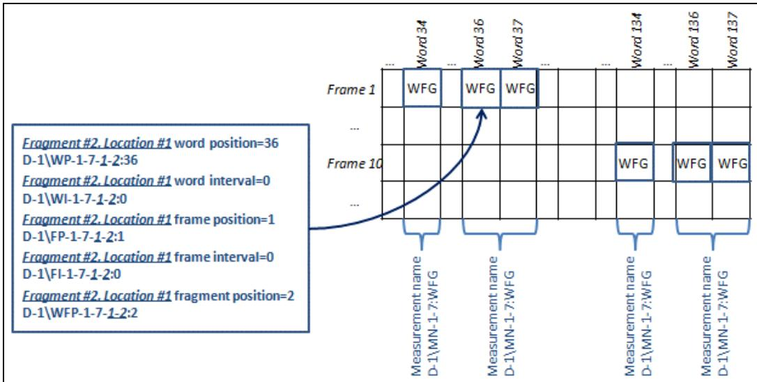
Figure 5-16. Subframe Fragmented Measurement in Multiple Locations
