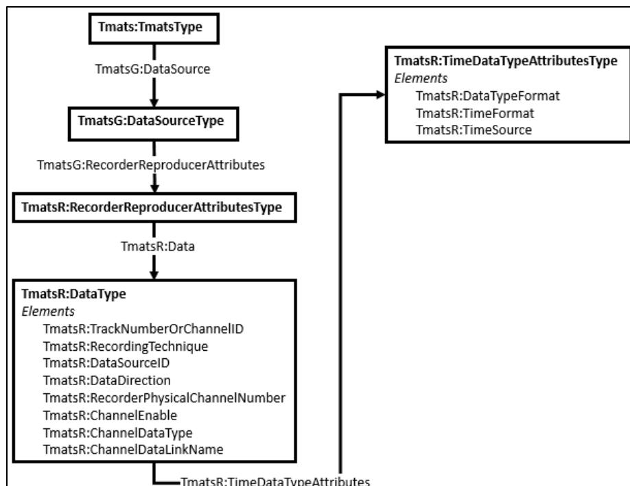
Figure 5-40. R-Group Sample Time Channel Example XML Schema
