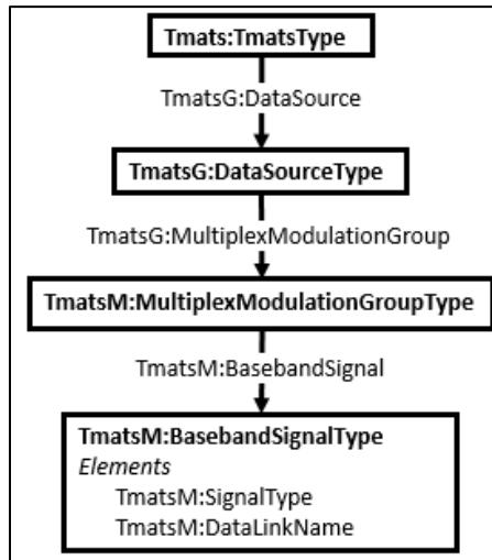
Figure 3-6. Multiplex/Modulation Attributes Group Example XML Schema
