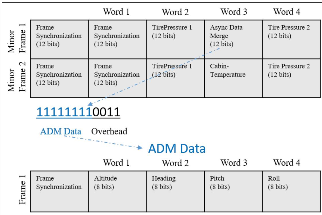
Figure 6-2. Simple Asynchronous Data Merge PCM Example
