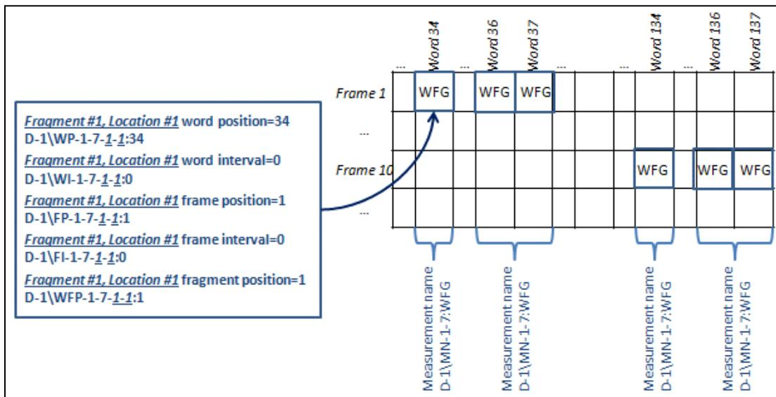
Figure 5-15. Subframe Fragmented Measurement in Multiple Locations
