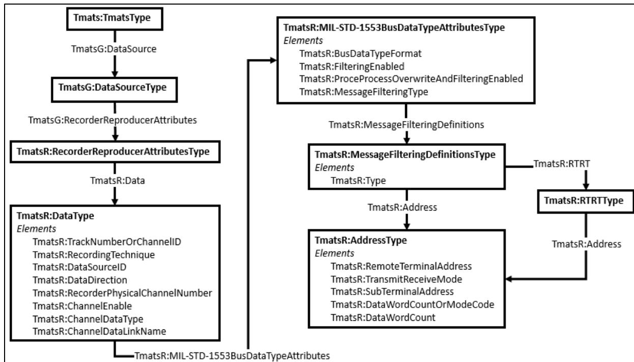
Figure 5-44. R-Group Sample 1553 Channel Example XML Schema
