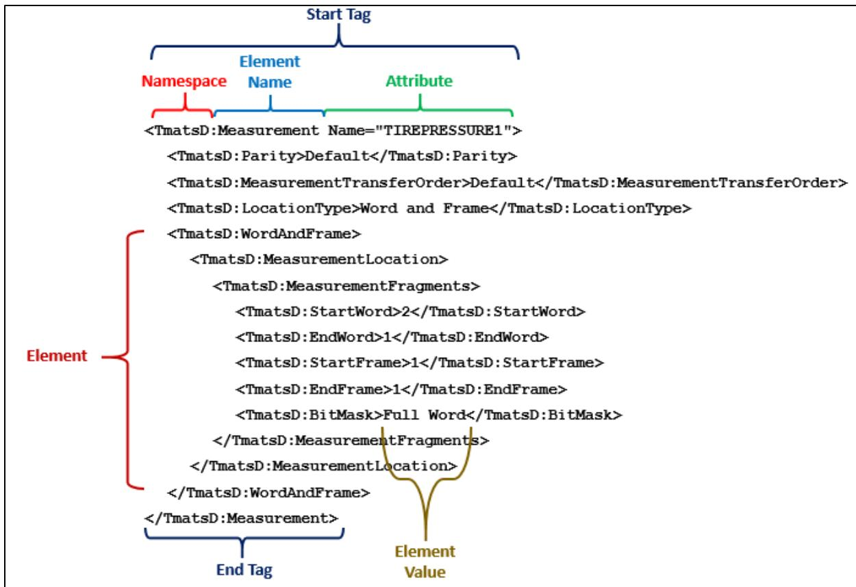
Figure 2-2. Components of an XML Element
