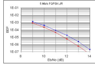
Figure 2-101. BEP versus  $E_b/N_0$  for FQPSK-JR.
