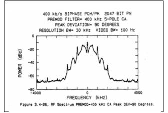
Figure 2-94. RF spectrum PREMOD = 400 kHz CA peak DEV = 90 Degrees.
