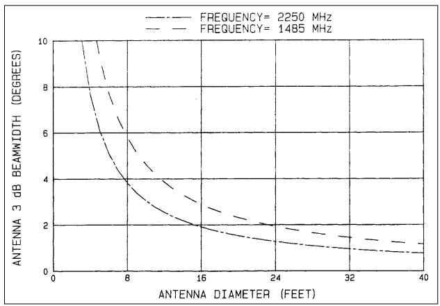
Figure 4-3. Antenna beamwidth versus diameter (50 percent efficiency).
