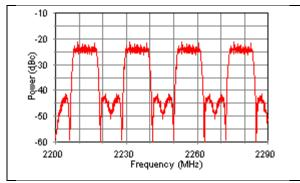
Figure 2-216. 10 Mb/s NRZ PCM/FM with receiver with typical RLC filters assumed.
