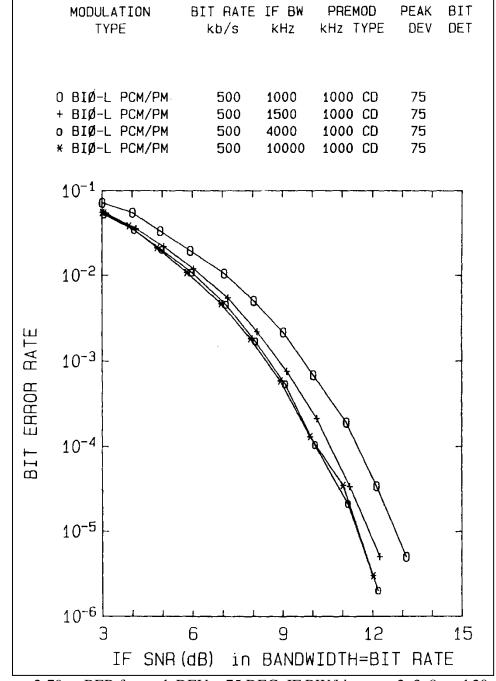
Figure 2-79. BER for peak DEV = 75 DEG, IF BW/bit rate = 2, 3, 8, and 20.
