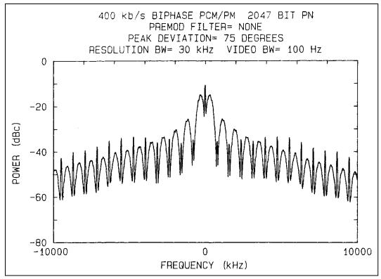
Figure 2-82. 400 kb/s biphase PCM/PM RF spectrum (20 MHz bandwidth).
