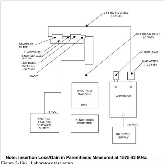
Figure 2-196. Laboratory test setup.
