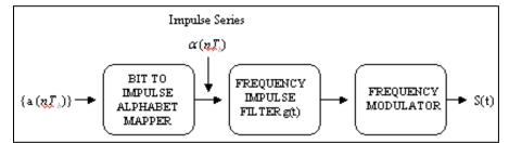
Figure 2-102. Basic SOQPSK block diagram.
