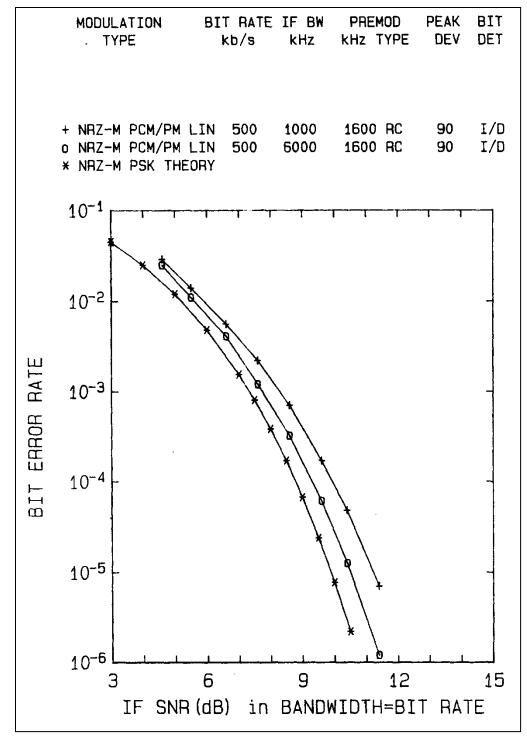
Figure 2-54. BER for IF BW/bit rate = 2 and 12.
