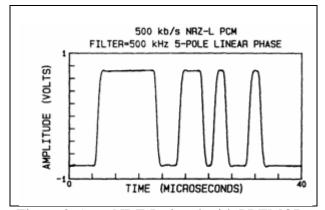
Figure 2-5. NRZ-L signal with PREMOD filter = bit rate.
