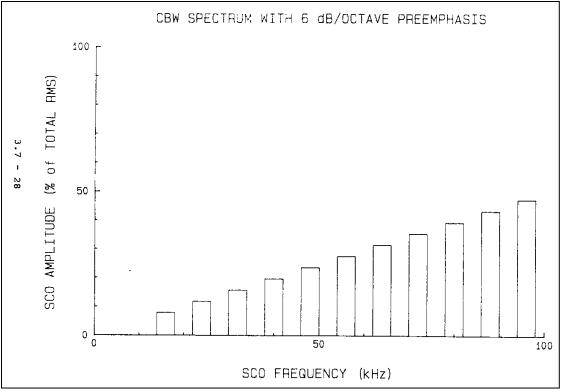
Figure 2-148. CBW spectrum with 6 dB/octave preemphasis.
