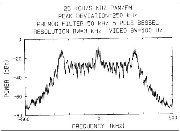
Figure 2-128. PAM/FM RF spectrum with peak deviation = 250 kHz.
