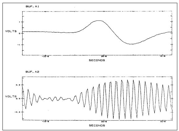
Figure 2-193. Doublet (upper trace) and IF signal.
