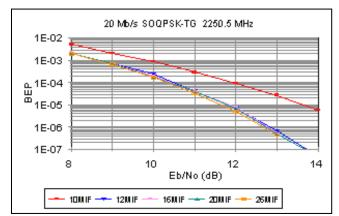
Figure 2-108. SOQPSK-TG BEP performance with various IF bandwidths.
