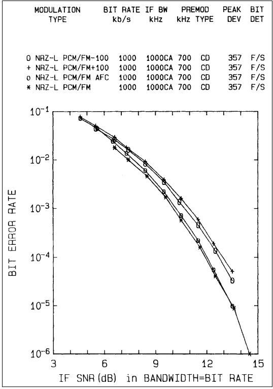
Figure 2-11. BER with AFC and with 100 kHz detuning.
