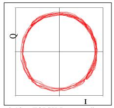
Figure 2-98. FQPSK-B vector diagram.
