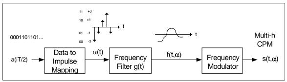
Figure 2-109. Conceptual CPM modulator.
