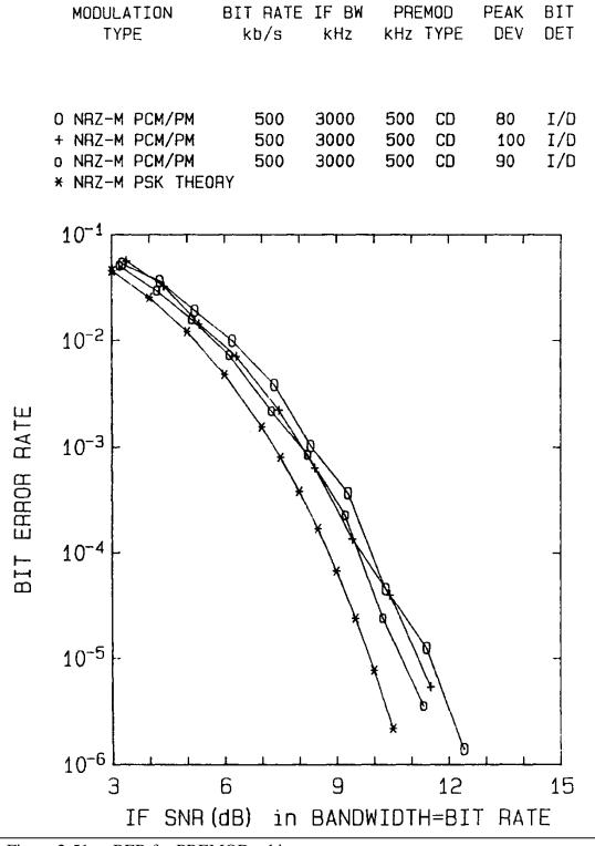
Figure 2-51. BER for PREMOD = bit rate.
