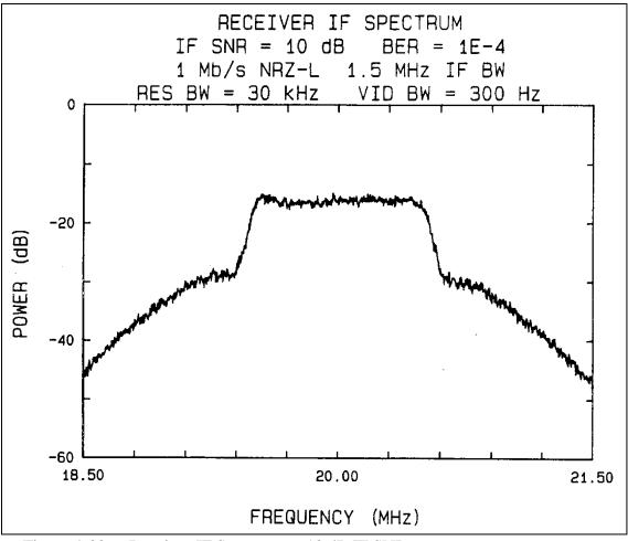
Figure 4-38. Receiver IF Spectrum at 10 dB IF SNR.
