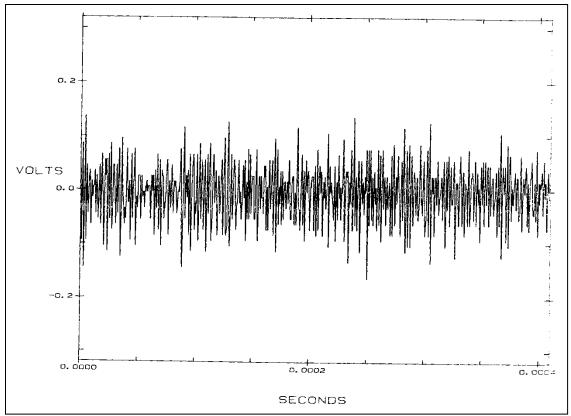
Figure 2-178. Fluctuation noise.
