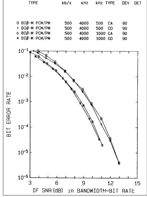
Figure 2-74. BER for peak DEV = 90 DEG and PREMOD = 1 and 2 bit rate.
