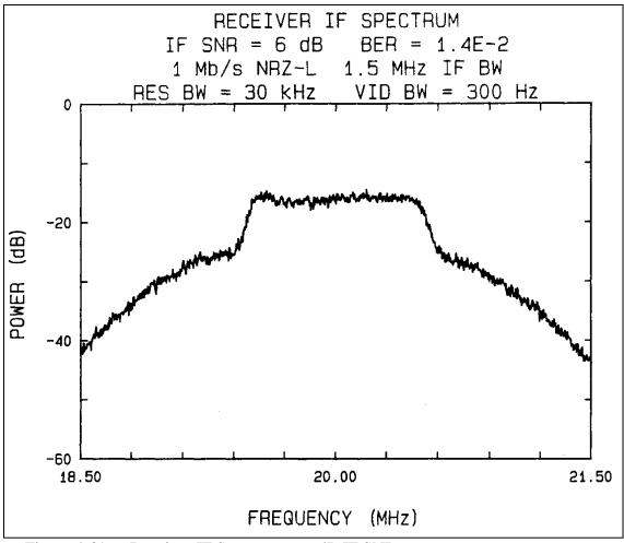
Figure 4-39. Receiver IF Spectrum at 6 dB IF SNR.
