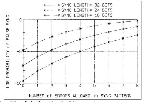
Figure 3-3. Probability of detecting false sync pattern.
