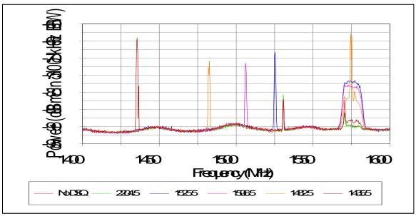
Figure 2-195. Spectrum analyzer plots at GPS LNA output.
