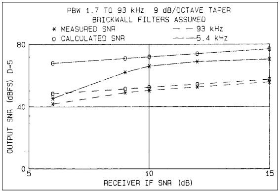
Figure 2-139. PMW measured and calculated SNRs with Brickwall Filters.
