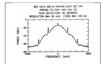
Figure 2-65. RF spectrum PREMOD = 400 kHz CD peak DEV = 90 degrees.
