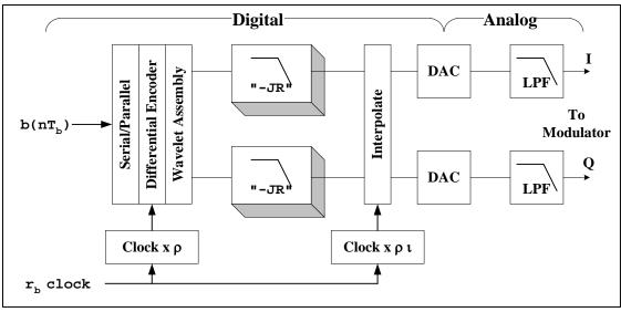
Figure 2-95. FQPSK-JR baseband signal generator.
