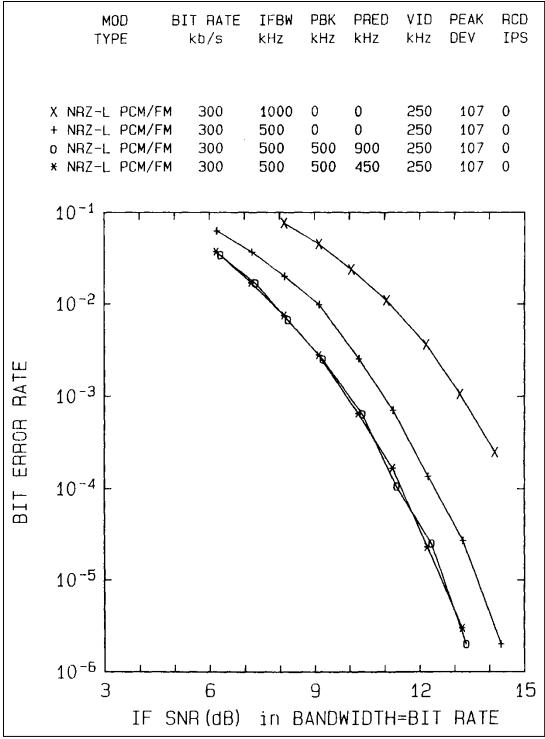
Figure 4-21. BER with 300 kb/s and 450 and 90 kHz PRE-D.
