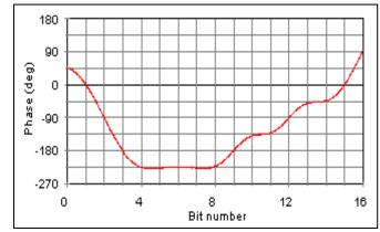
Figure 2-104. Measured SOQPSK-TG phase trajectory.
