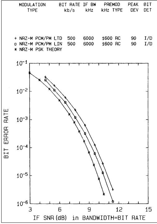
Figure 2-55. BER for linear and limited IF signals.
