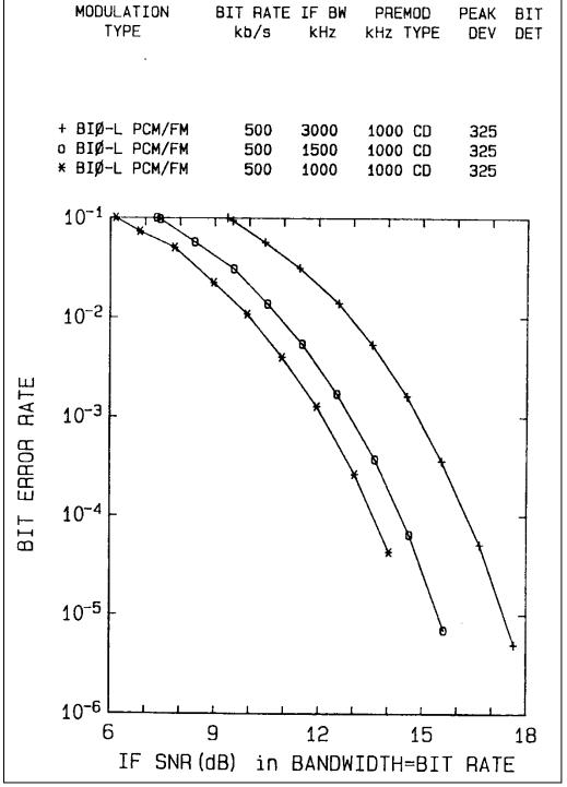
Figure 2-42. BER for IF BW/bit rate = 2, 3, and 6.
