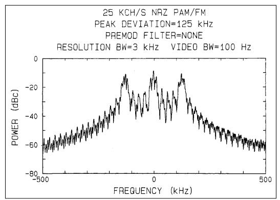
Figure 2-129. PAM/FM RF spectrum with No Premodulation Filter.
