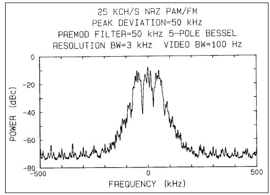
Figure 2-126. PAM/FM RF spectrum with peak deviation = 50 kHz.
