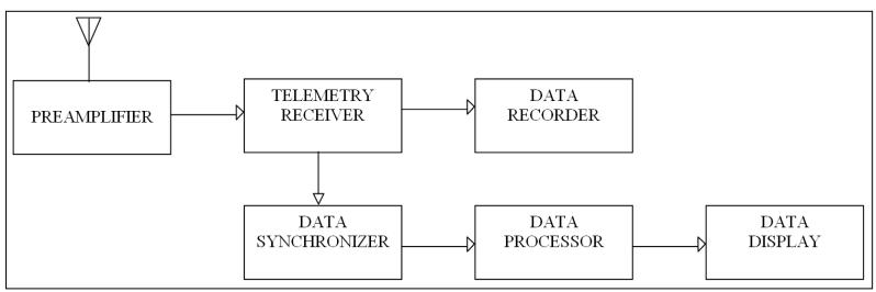
Figure 1-2. Telemetry receiving system.
