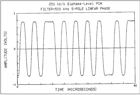
Biphase Signal with PREMOD BW = 2 times bit rate (CD). Figure 2-76.
