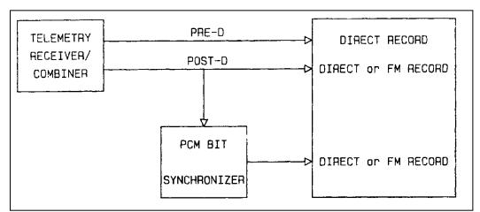
Figure 4-20. Methods for recording telemetry signals.
