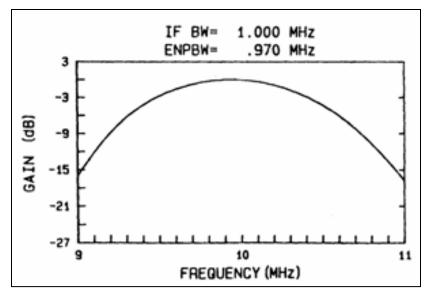
Figure 2-176. IF filter frequency response (Filter B).
