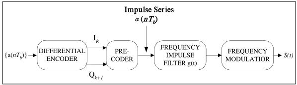
Figure 2-103. SOQPSK transmitter.
