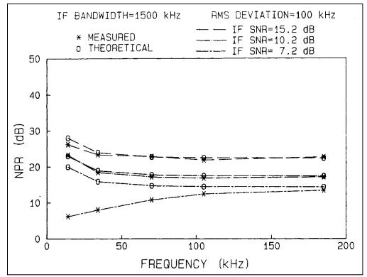
Figure 2-162. Measured and theoretical NPRs (1500 kHz IF, 100 kHz deviation).
