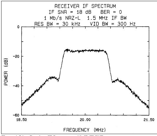
Figure 4-36. Receiver IF Spectrum at 18 dB IF SNR.
