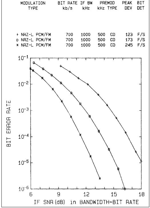
Figure 2-4. BER for peak DEV/bit rate = 0.175, 0.25, and 0.35.
