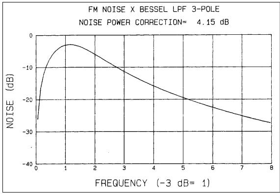
Figure 2-133. FM Noise with 3-pole Bessel LPF.
