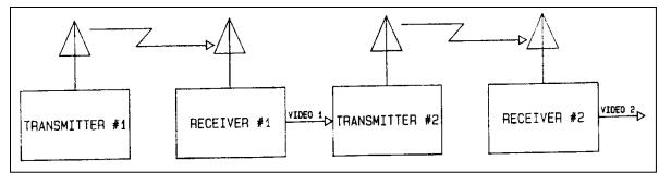
Figure 2-171. Block diagram of demodulation/remodulation relay link.
