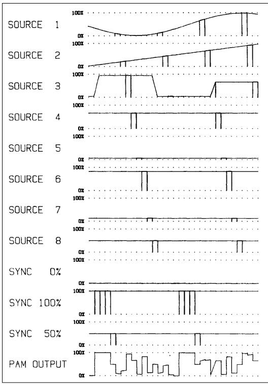
Figure 2-113. NRZ PAM Signal with Natural Sampling.
