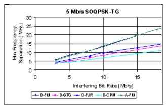
Figure 2-214. Minimum frequency separation.
