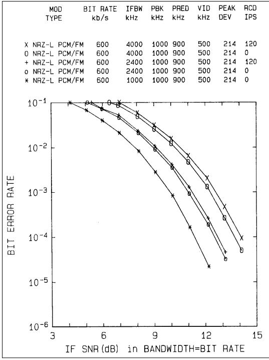
Figure 4-22. BER with and without recording.
