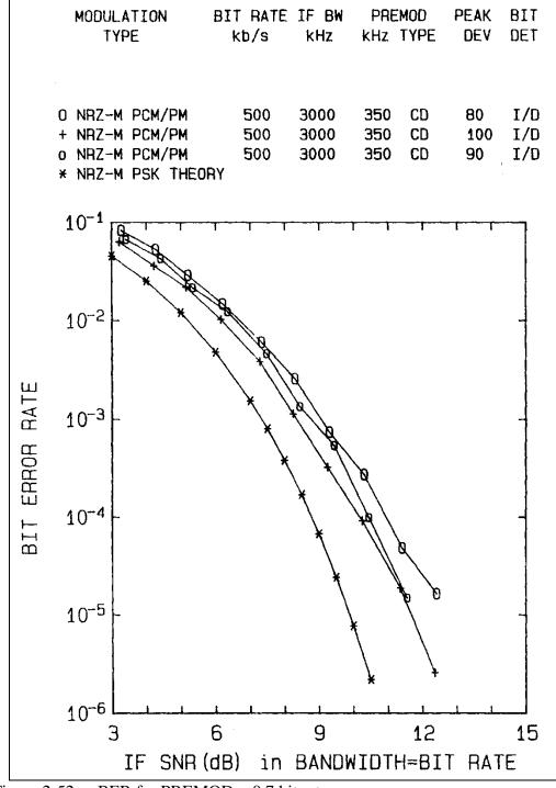
Figure 2-52. BER for PREMOD = 0.7 bit rate.
