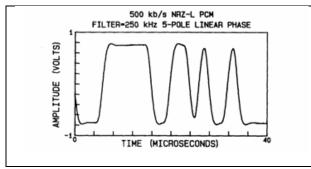
Figure 2-7. NRZ-L signal with PREMOD filter = bit rate/2 (CD).
