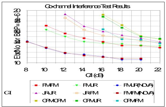
Figure 2-220. Co-channel interference test results.
