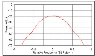
Figure 2-105. SOQPSK-TG power spectrum (5 mb/s).
