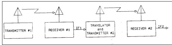
Figure 2-170. Block diagram of translation relay link.
