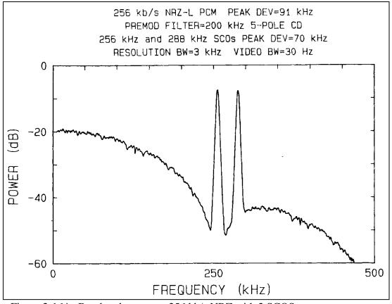
Figure 2-164. Baseband spectrum 256 kb/s NRZ with 2 SCOSs.
