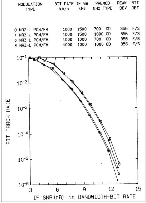
Figure 2-14. BER with IF BW bit rate = 1 and 1.5.
