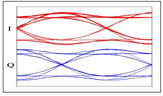
Figure 2-96. FQPSK wavelet eye diagram.
