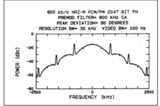
Figure 2-67. RF spectrum PREMOD = 800 kHz CA peak DEV = 90 degrees.
