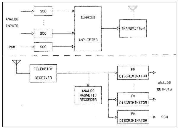
Figure 2-131. FM/FM system block diagram.
