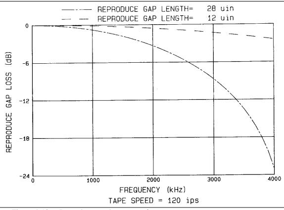
Figure 4-13. Reproduce gap loss versus frequency.
