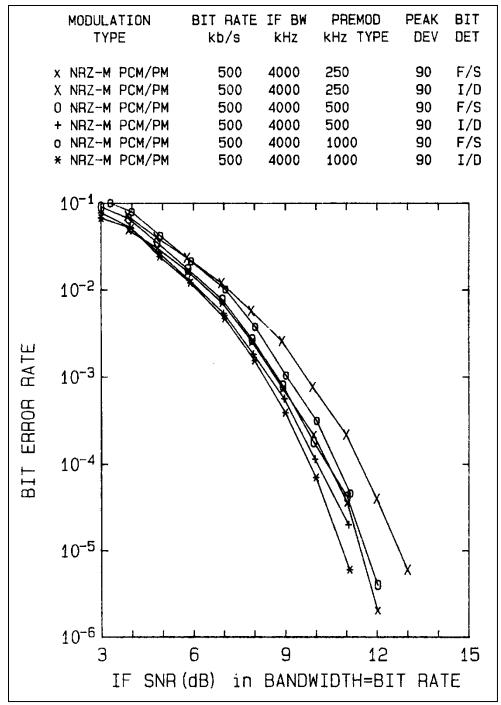
Figure 2-56. BER for video BW/BIT rate = 0.5, 1, and 2.
