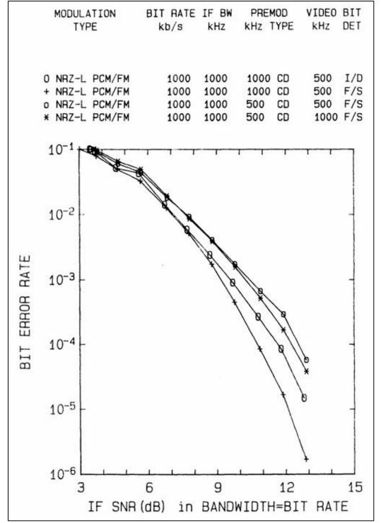
Figure 2-15. BER with video and PREMOD BWs = 0.5 and 1 bit rate.
