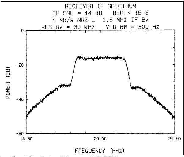
Figure 4-37. Receiver IF Spectrum at 14 dB IF SNR.
