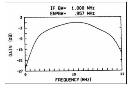
Figure 2-177. IF filter frequency response (Filter C).
