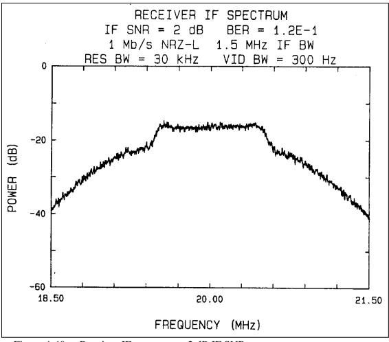
Figure 4-40. Receiver IF spectrum at 2 dB IF SNR.
