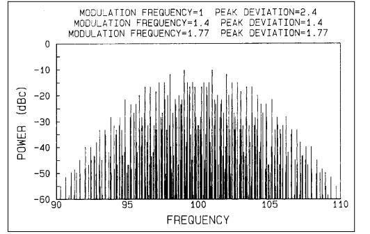
Figure 2-157. FM spectrum with three sine wave modulation and MI = 1 and MI = 2.4.
