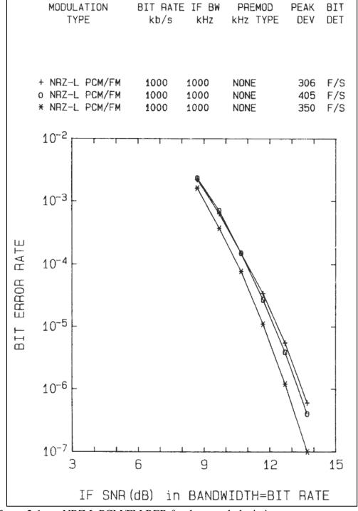
Figure 2-1. NRZ-L PCM/FM BER for three peak deviations.
