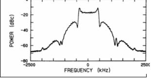
Figure 2-23. RF spectrum PREMOD = 800 kHz CD peak DEV = 0.42 bit rate.
