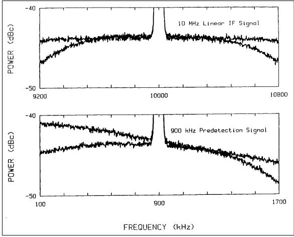
Figure 4-24. Noise PSDs for IF and PRE-D signals.
