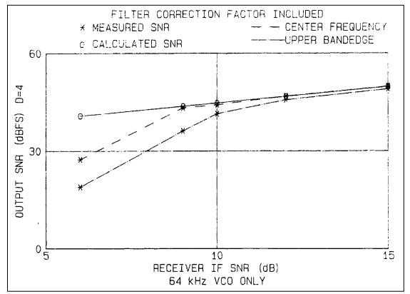
Figure 2-144. Measured and calculated SNRs with correction factors (D = 4).
