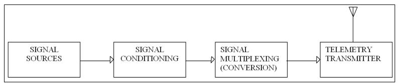
Figure 1-1. Telemetry transmitting system.
