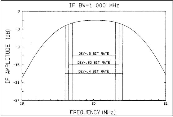
Figure 2-3. IF filter attenuation versus peak deviation.
