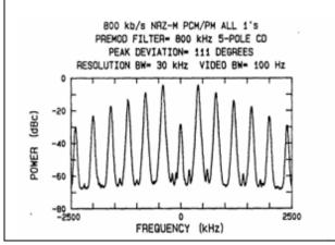
Figure 2-63. RF spectrum PREMOD = 800 kHz CD peak DEV = 111 degrees (1s).
