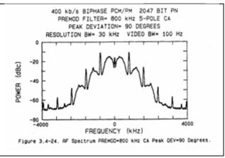
Figure 2-92. RF spectrum PREMOD = 800 kHz CA peak DEV = 90 degrees.
