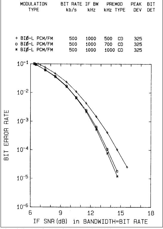
Figure 2-40. BER for PREMOD BW = 1, 1.4, and 2 bit rate.
