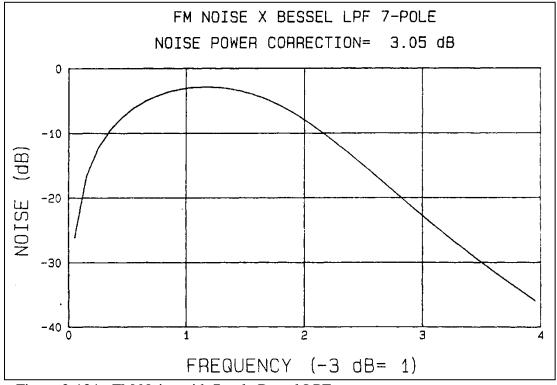
Figure 2-134. FM Noise with 7-pole Bessel LPF.
