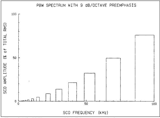
Figure 2-150. PBW spectrum with 9 dB/octave preemphasis.
