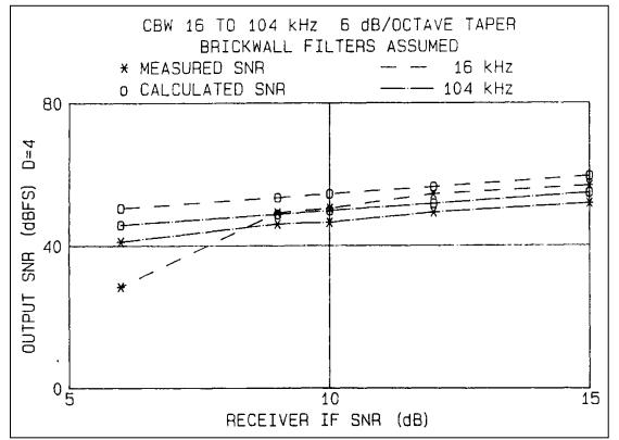
Figure 2-140. CBW measured and calculated SNRs with Brickwall Filters.
