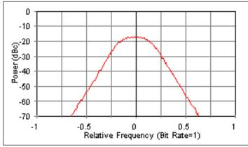
Figure 2-110. Power spectrum of 5 MB/S ARTM CPM.
