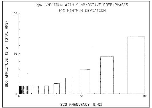
Figure 2-151. PBW spectrum with 9 dB/octave preemphasis and 10 percent minimum amplitude.
