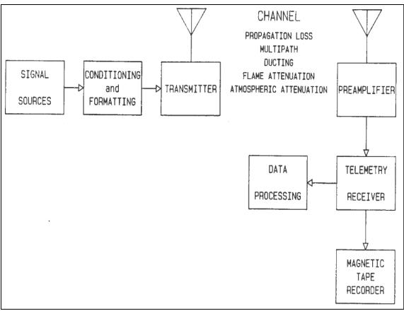
Figure 2-167. Block diagram of telemetry link.
