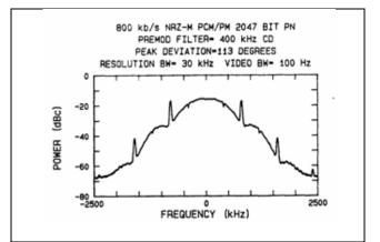
Figure 2-66. RF spectrum PREMOD = 400 kHz CD peak DEV = 113 degrees.
