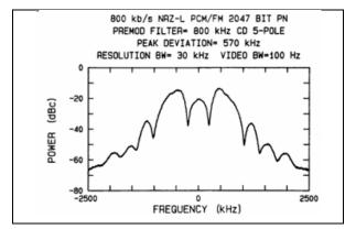
Figure 2-25. RF spectrum PREMOD = 800 kHz CD peak DEV = 0.71 bit rate.
