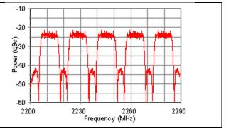
Figure 2-217. 10 Mb/s NRZ PCM/FM with multi-symbol detector assumed.
