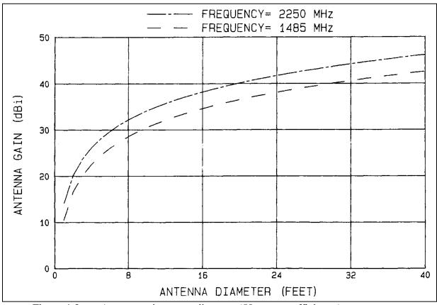
Figure 4-2. Antenna gain versus diameter (50 percent efficiency).
