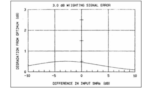
Figure 4-8. Combiner degradation from optimum with 3 dB weighting error.
