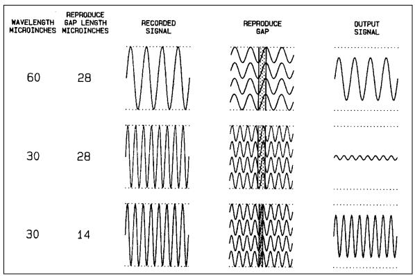
Figure 4-12. Reproduce gap loss illustration.
