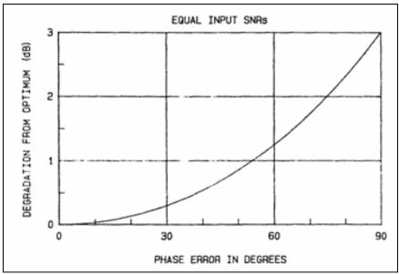
Figure 4-9. Combiner degradation from optimum versus phase error.
