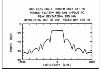
Figure 2-33. RF spectrum PREMOD = 560 kHz RC peak DEV = 0.35 bit rate.
