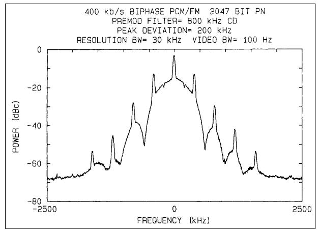
Figure 2-44. Biphase PCM/FM RF spectrum (PREMOD=800 kHz CD, DEV=0.50 bit rate).
