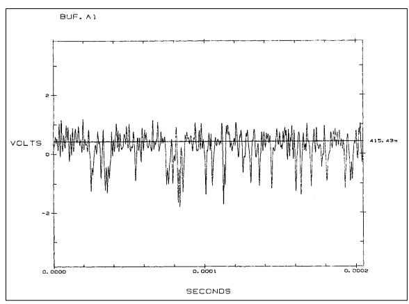
Figure 2-185. Pop noise with IF signal = 10.25 MHz.
