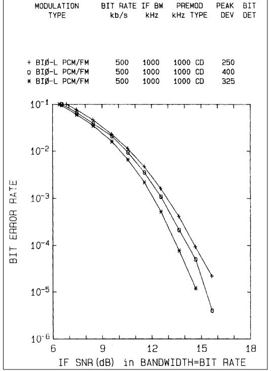
Figure 2-38. BER for peak DEV = 0.5, 0.65, and 0.8 bit rate for IF BW = 2 times bit rate.
