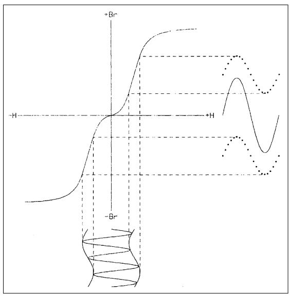
Figure 4-16. Recording with ac-bias.
