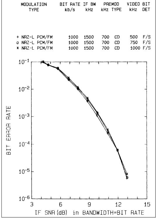
Figure 2-17. BER with video BW = 0.5, 0.75, and 1 bit rate.
