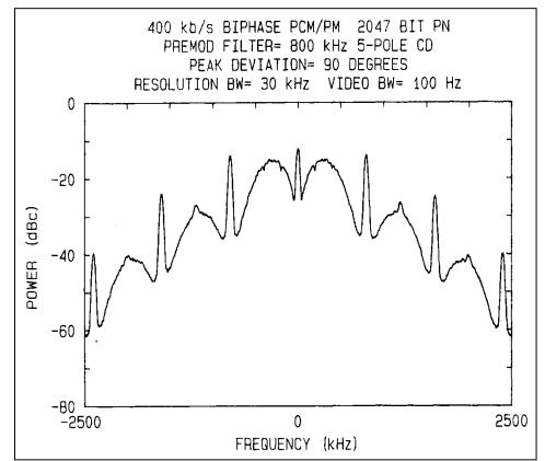
Figure 2-69. 400 kb/s biphase PCM/PM RF spectrum (PREMOD = 800 kHz CD, DEV = 90 degrees.
