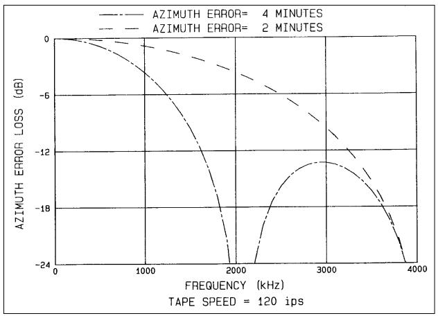
Figure 4-11. Azimuth error loss versus frequency (120 ips).
