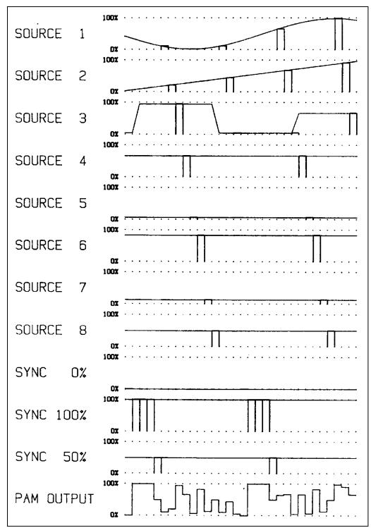
Figure 2-112. NRZ PAM signal with flat-top sampling.
