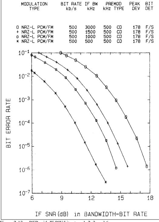
Figure 2-13. BER with IF BW/bit rate = 1, 2, 3, and 6.
