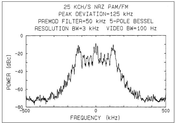
Figure 2-127. PAM/FM RF spectrum with peak deviation = 125 kHz.
