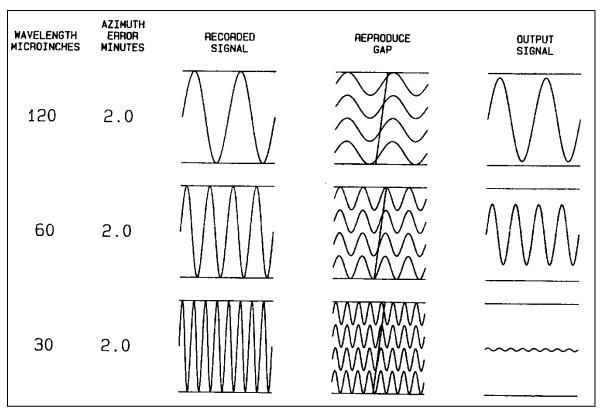
Figure 4-10. Azimuth error illustration.
