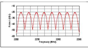
Figure 2-218. 10 Mb/s SOQPSK-TG or FQPSK-JR.
