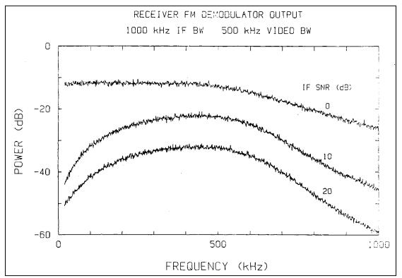
Figure 2-179. Receiver video noise power spectral density.
