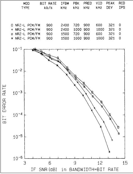
Figure 4-26. Upconversion versus tape carrier demodulation.
