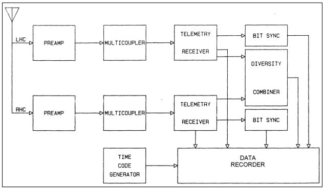
Figure 4-1. Simplified telemetry receive/record station.
