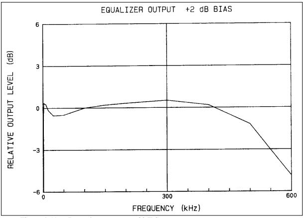
Figure 4-19. Reproducer output at 30 IPS.
