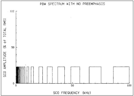
Figure 2-149. PBW spectrum with no preemphasis.
