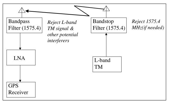
Figure 2-201. Block diagram of L-band telemetry and GPS systems designed to minimize interference.
