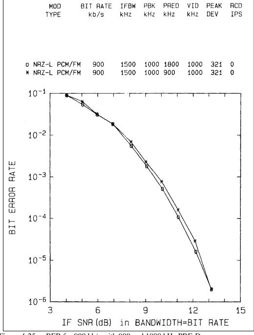
Figure 4-25. BER for 900 kb/s with 900 and 1800 kHz PRE-D.
