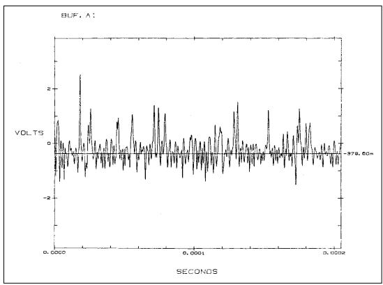
Figure 2-186. Pop noise with IF signal = 9.75 MHz.
