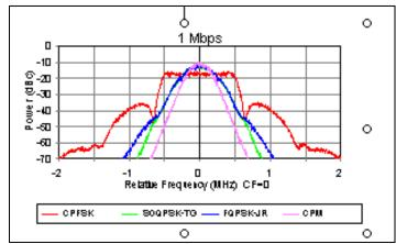
Figure 2-203. Signal spectra.
