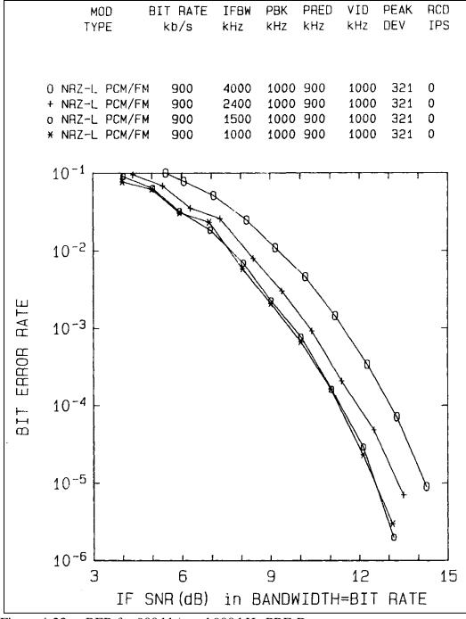
Figure 4-23. BER for 900 kb/s and 900 kHz PRE-D.
