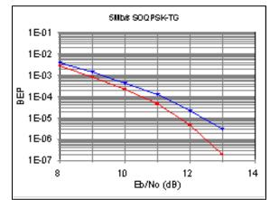
Figure 2-106. BEP versus Eb/No performance of 5 Mb/s SOQPSK-TG.
