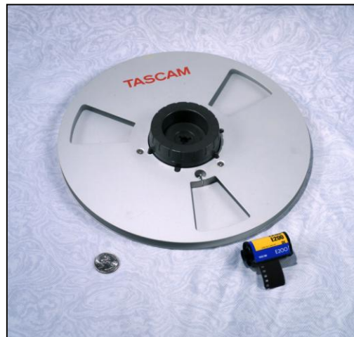
Figure 1-1. 1/2 inch open reel videotape.
