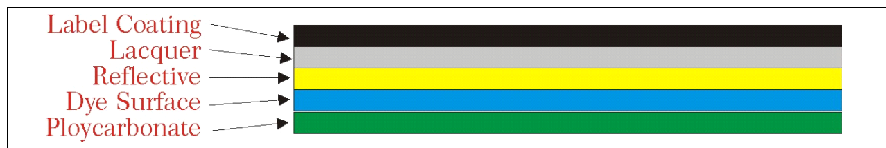
Figure 2-4. Five-layer structure of recordable discs.
